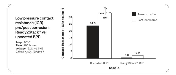
Corrosion test conditions: pH2.8 @ 2.2Vx100h, Ti - grade 1
